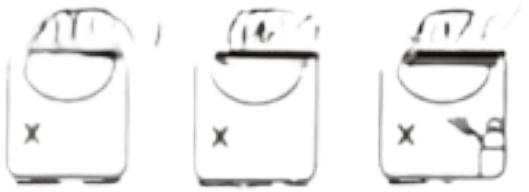
Unstable ceilings Open-air places High temperature and humid areas
