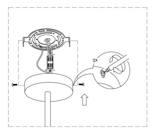
The side screws fix the lamp body to the ceiling plate
