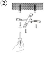
2. Fix the pegboard inside the expansion tube of the ceiling with self-tapping screws and lock the across pegboard tightly with a screwdriver.
