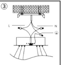
3. Connect the wires in the ceiling and the lamps with zero wire and zero wire.fire wire and fire wire earth wire and earth wire, respectively, and then tighten the wires with wiring caps and tie them with ties.
