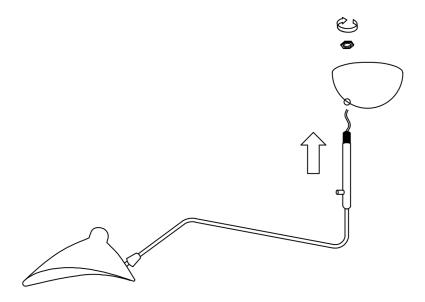
The lamp body and ceiling tray are fixed together with screws
