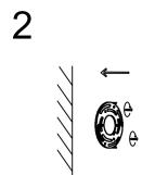
Install the hanging plate on the wall
