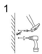
Drill holes in the wall and insert expansion screws
