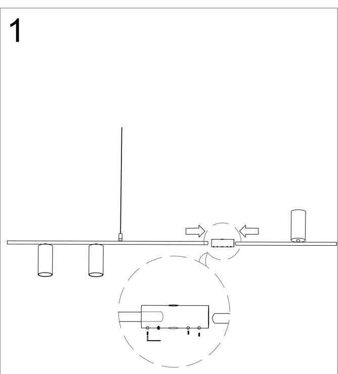
Insert the tube and then fix it with a few screws, the same at both ends
