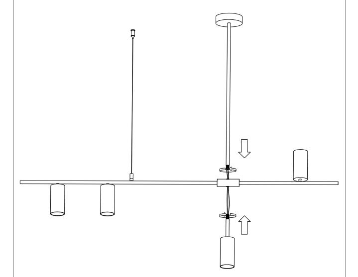
After inserting the wire, twist it into the lamp body
