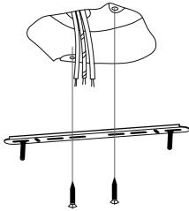
Fasten the hanging board to the ceiling with screws
