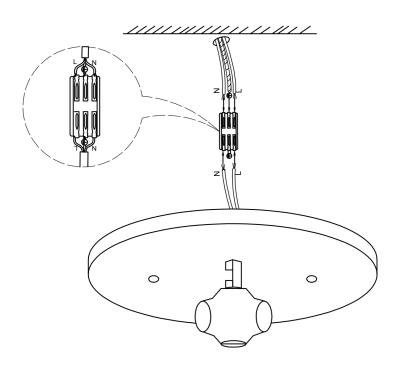
The wires in the home are connected to the wires in the lamps through the wire terminals
