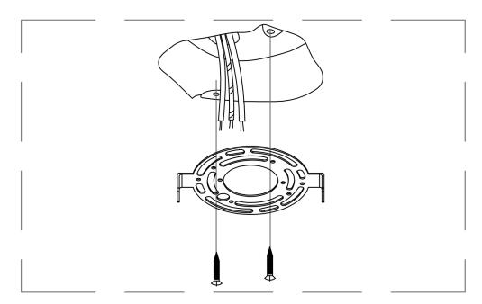
Fasten the hanging board to the ceiling with screws
