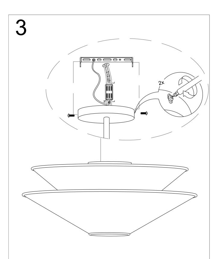
The side screws fix the lamp body to the ceiling plate
