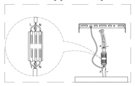
The wires in the home are connected to the wires in the lamps through the wire terminals
