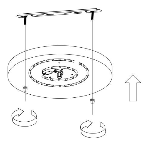
Use hand-made nuts to fix the lamp body on the hanging board
