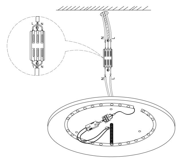
The wires in the home are connected to the wires in the lamps through the wire terminals
