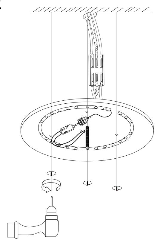
Fasten the hanging board to the ceiling with screws
