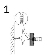
The home wire is connected to the lamp wire
