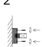
Screw the top plate to the wall
