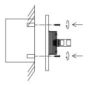
Screw the top plate to the wall
