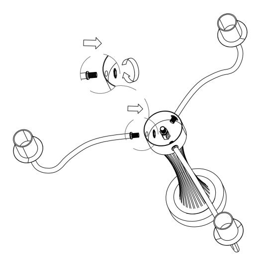
Use screws to lock the lamp arm onto the lamp body
