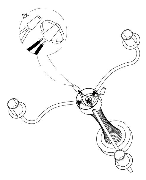
The main line is connected to the wires of the same color
