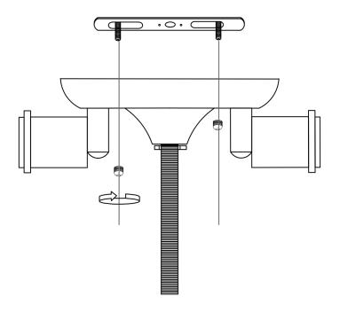
Use hand-made nuts to lock the lamp body on the hanging plate
