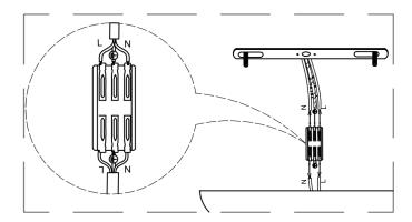
The wires in the home are connected to the wires in the lamps through the wire terminals
