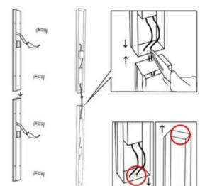
Single lamp installation The dotted line of the reserved wiring must be installed in the downward
