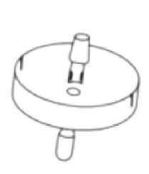
3. Adjust the length of the wire until the appropriate length. (if the lamp wire is long can be properly cut off) Then connect the fire wire zero wire to the fixture's fire wire zero wire.
