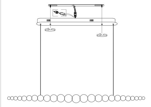
Use hand-made nuts to fix the lamp body on the hanging board
