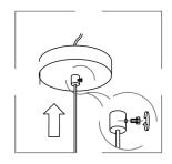
After adjusting the line length, fix it with screws.
