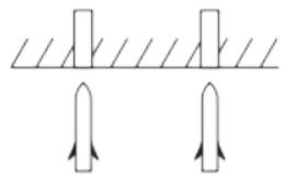
1. Use a drill bit to estimate two holes in the ceiling. Align the holeswith the pegboard holes, and then hammer them into the wall with expansion screws.
