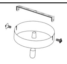
4. Use the small screws in the kit in the side of the seat plate to fix the chassis and hanging plate
