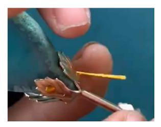
Insert the onyx piece into the hole, then press the pin
