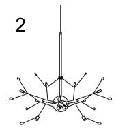
The lamp arm wire is connected to the main line
