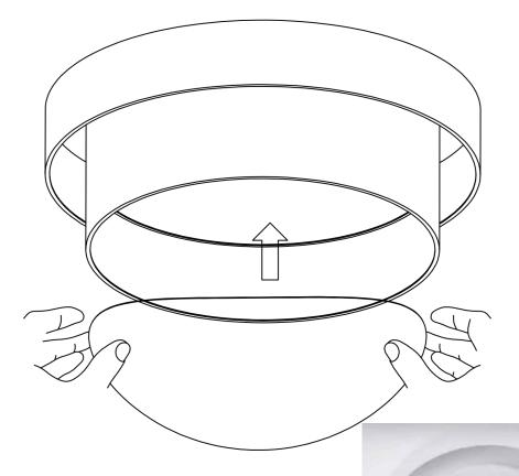
The acrylic bends a small arc and stuffs it into the lamp body
