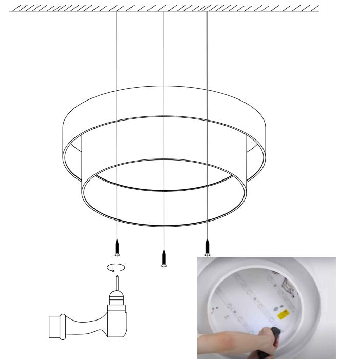
After the wires are connected, use screws to lock the lamp body to the ceiling.
