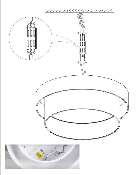
The wires in the home are connected to the wires in the lamps through the wire terminals
