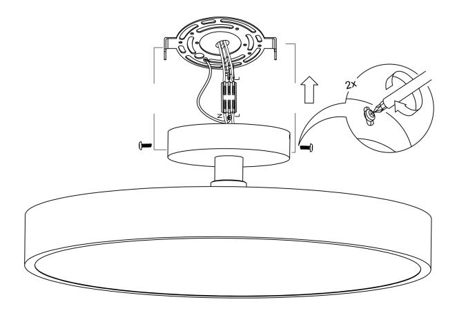
The side screws fix the lamp body to the ceiling plate
