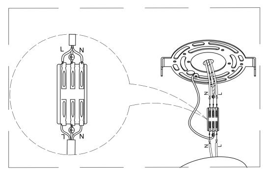
The wires in the home are connected to the wires in the lamps through the wire terminals
