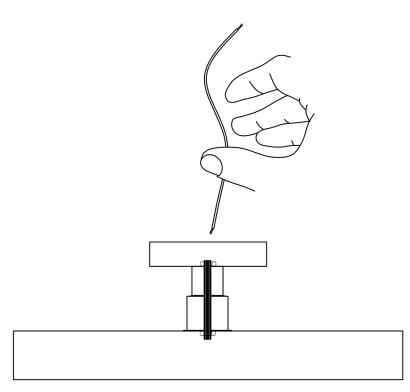
Insert the main line and connect it to the internal terminal
