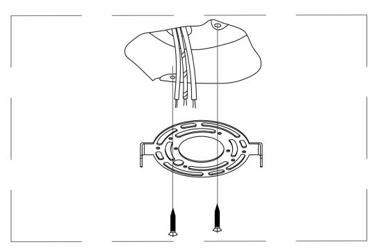
Fasten the hanging board to the ceiling with screws
