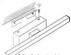
3. Use the hanging plate screws to tighten the lamp and the hanging plate from above.
