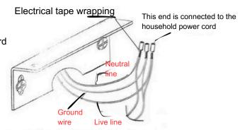
2. Connect the reserved wires to the lamp drive wires
