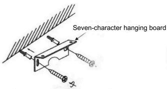
1.Fix the hanging board to the wall with self-tapping screw expansion caps
