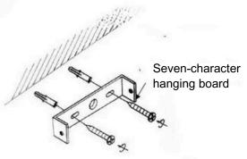
1.Fix the hanging board to the wall with self-tapping screw expansion caps
