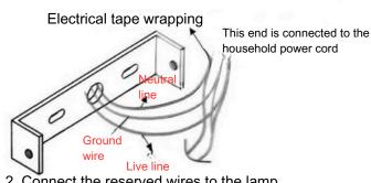
2. Connect the reserved wires to the lamp drive wires
